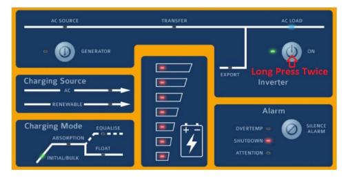
4. Wait until Low DC shutdown recovers. When the battery LEDs stop flashing red and the SP PRO remains on then the system has recovered.
